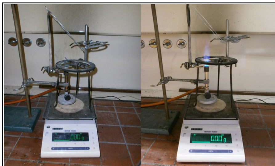
Fig. 2. The testing device for fire tests constructed and located in the Fire-chemical laboratory of the Department of Fire Engineering, Faculty of Security Engineering, University of Zilina
