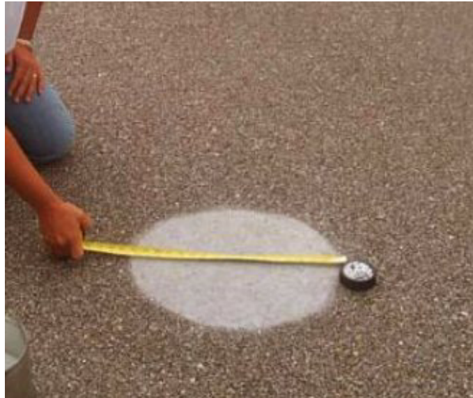
Fig. 2. Measurement of texture - the sand patch test
