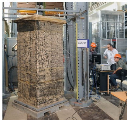
Fig. 2: Geosynthetic reinforced soil laboratory specimen during loading test
