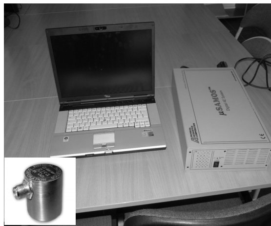
Fig. 3. The AE measuring set: 24 channels processor \mu SAMOS and resonance sensor with the frequency of 55 kHz [3-5].
