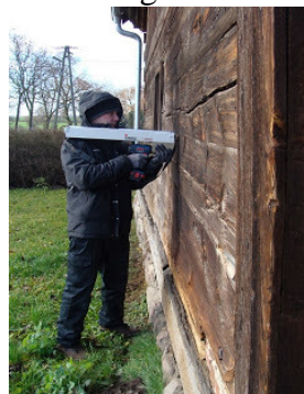
Fig. 3. Evaluation of wood condition with resistograph [12].
