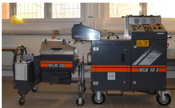
Fig. 2. Wirtgen WLB 10S laboratory foaming plant [J. Mrugała].
