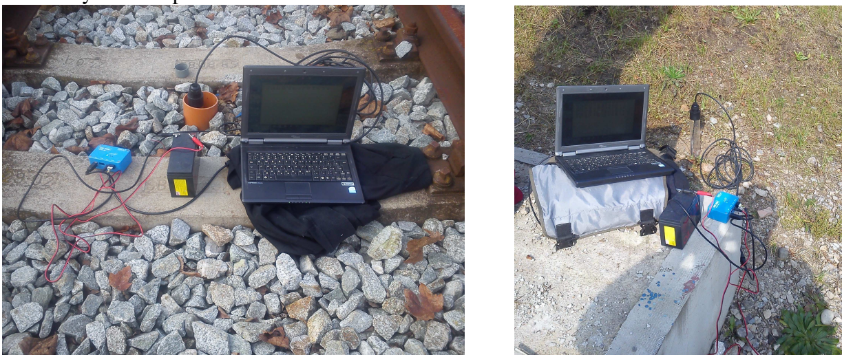
Fig. 3. Measurement of moisture content of structural layers (left) and subgrade (right) of the Experimental stand DRETM II.
