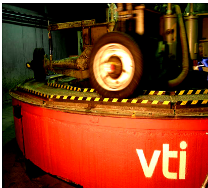
Fig. 5. The VTI road simulator and examples of measured results with APS [8].
