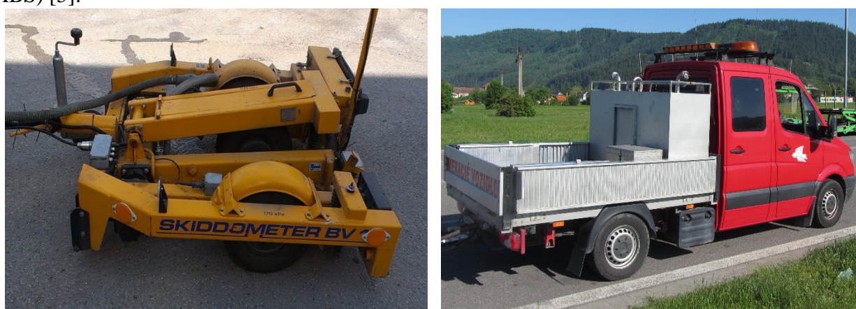
Fig. 3. Skiddometer BV11 together with towing vehicle.
