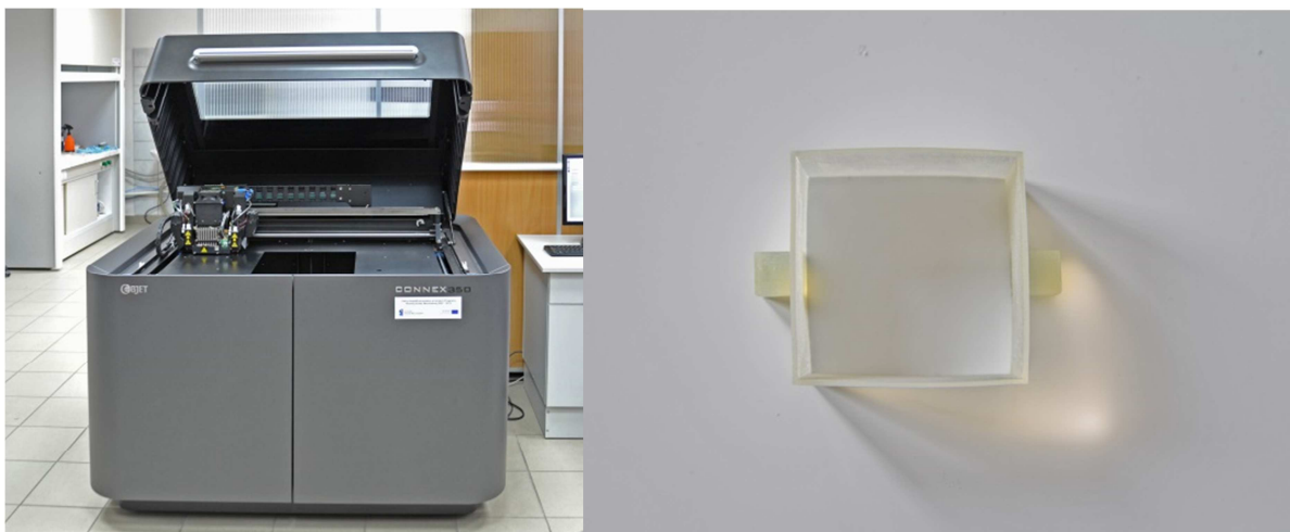
Fig. 2. Objet Connex 350 Printer and the manufactured thin wall cube model.
