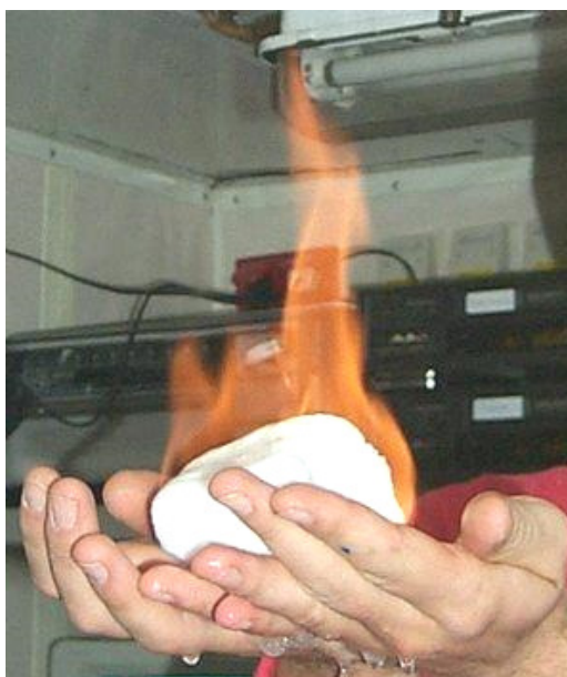
Fig. 3. Methane hydrate know also as “burning ice”.
