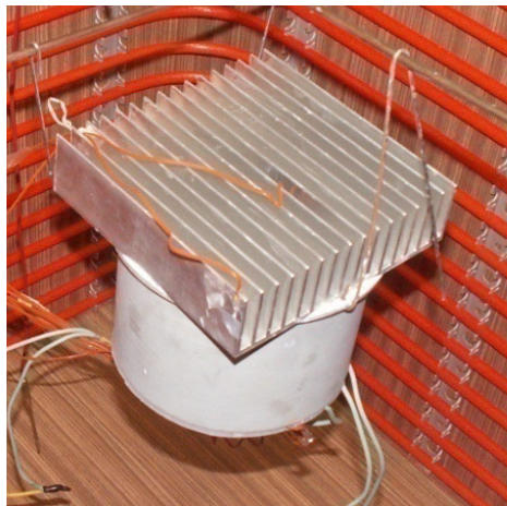
Fig. 4 Model of electrostatic converter with cooler.
