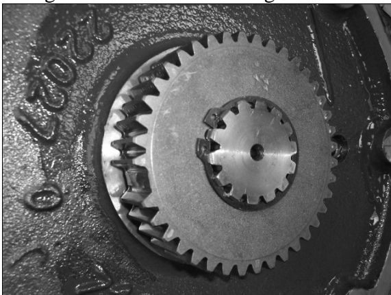
Fig. 2. Damaged sun gear with one missing tooth.
