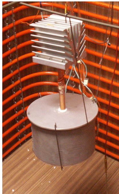
Fig. 5 Model of electrostatic converter with heat pipe.
