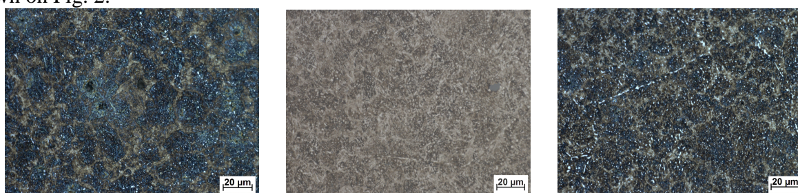
Fig. 2. Microstructures after heat treatment: a) martensitic, b) bainitic, c) sorbitic.
