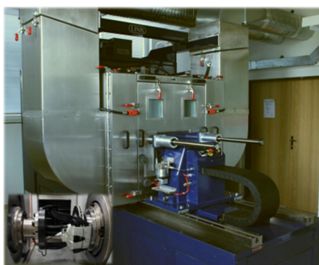
Fig. 1. Testing dynamometer of frictional properties of vehicular brake pads (Link M2800).
