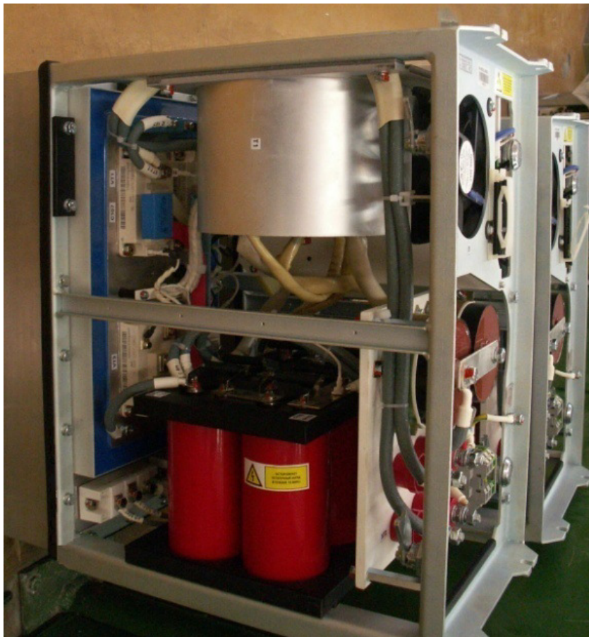
Fig. 1 Location of the transformer in the machine housing.
