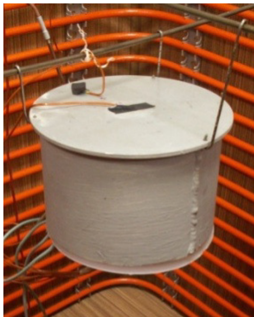
Fig. 3 Model of electrostatic converter without cooler.
