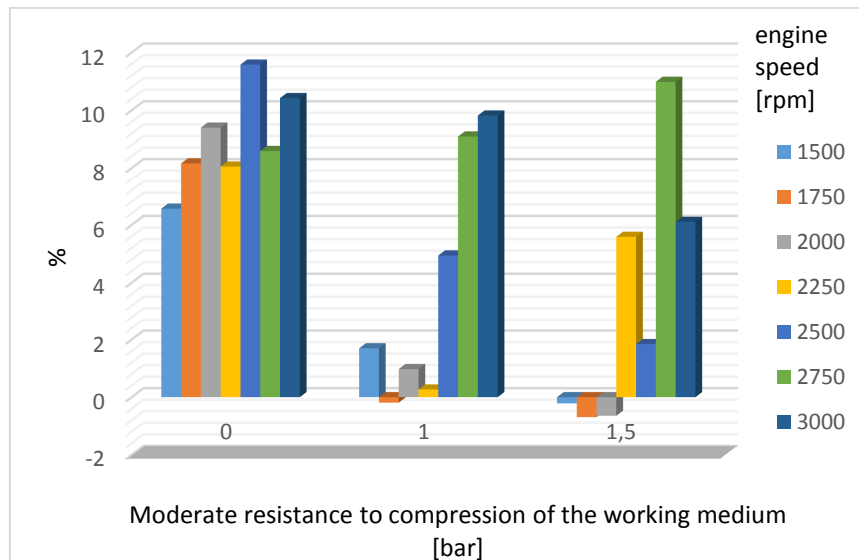
Fig. 2. Reduction of the loss of friction at different engine's revolution speed, temp of 80 °C
