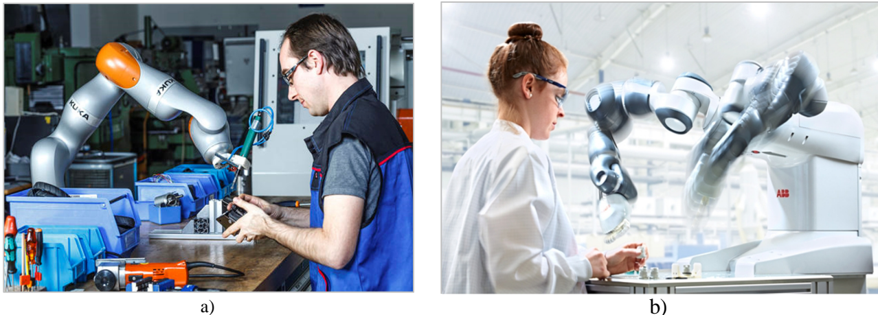
Fig. 2. Examples of application of cooperating robots in industry. a) KUKA iiwa, b) ABB YuMi.
