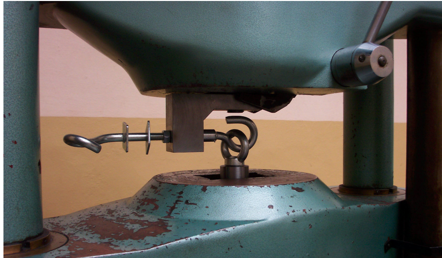
Fig. 2. Nut hook M16 during the bending tests F_Y , hook-thread type.
