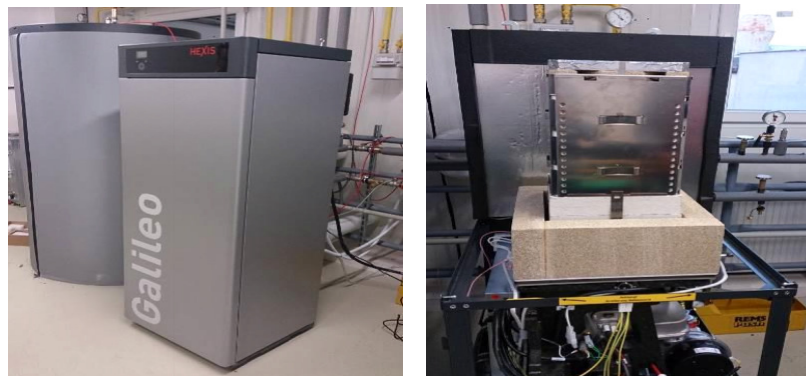
Fig. 1 SOFC Hexis Galileo 1000N and look inside of the fuel cell unit
