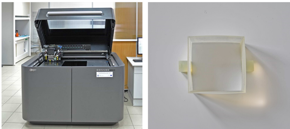
Fig. 2. Objet Connex 350 Printer and the manufactured thin wall cube model.
