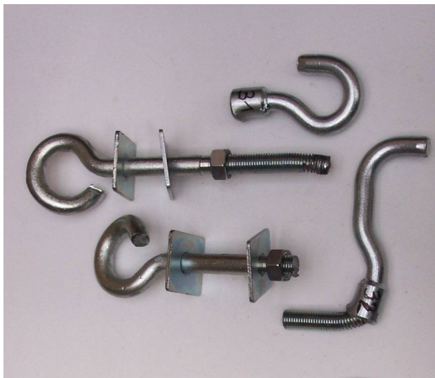
Fig.7. Nut hook M20 after the bending tests F_Y , hook-thread type.
