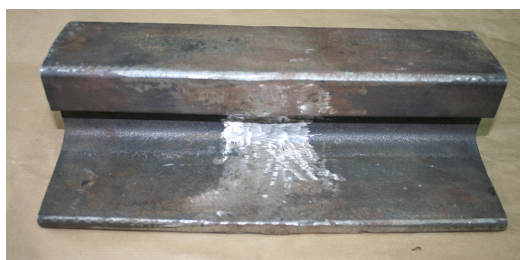
Fig. 2. Experimental welded joint of bridge rail
