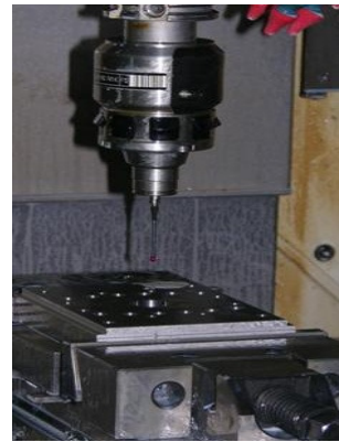
Fig. 2. The workpiece settings by touch probe.
