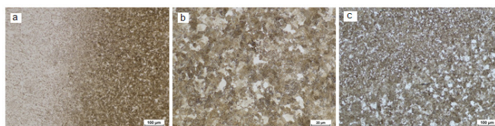
Fig. 7. The microstructure in points a-c (a – line of fusion, b – coarse grain zone, c – contrast between the base material and the heat affected zone)
