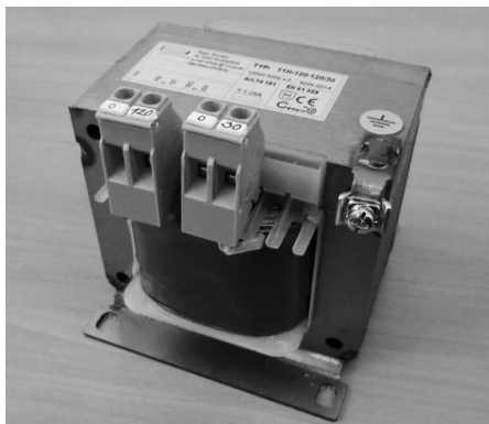
Fig. 2. Single-phase injection transformer - booster for DVR model
