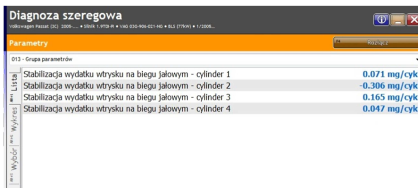
Fig.4. CDIF2 Diagnostic Program window – fuel injection dose stabilisation parameters readout [author's own material]
