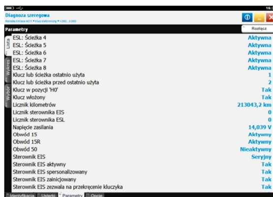
Fig .7 . CDIF3 Diagnostic Program window – Actual parameters of the key module readout vehicle MB W211 [author's own material]
