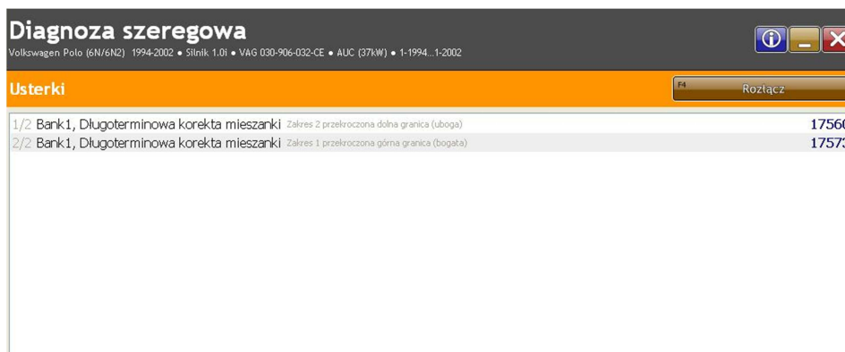
Fig.6. CDIF2 Diagnostic Program window – reaction time exceeded failure of the lambda probe [author's own material]
