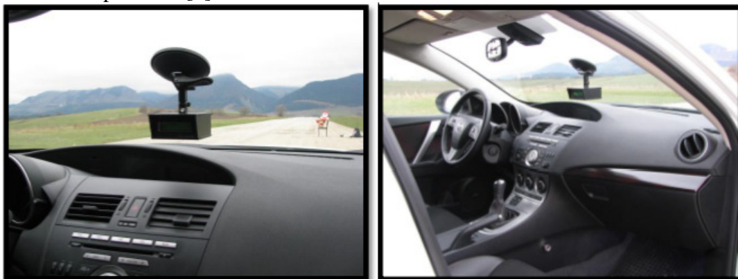
Fig. 3. Location of XL Meter TM Pro in the vehicle
