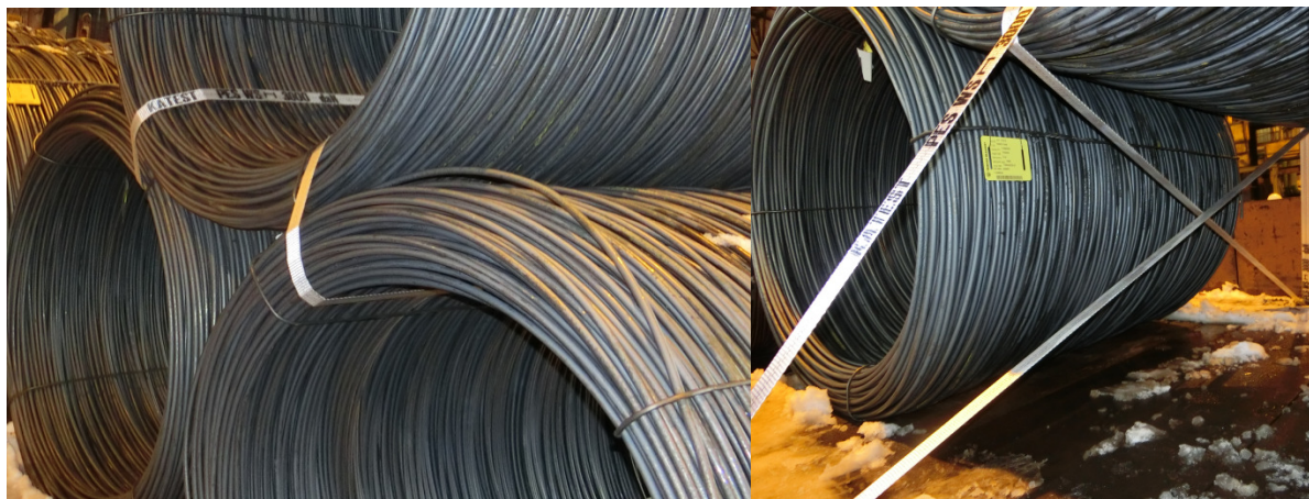
Fig. 1 Securing of the coil in upper layer in the first series of impact tests (in the left) and in the second series of impact tests (in the right)
