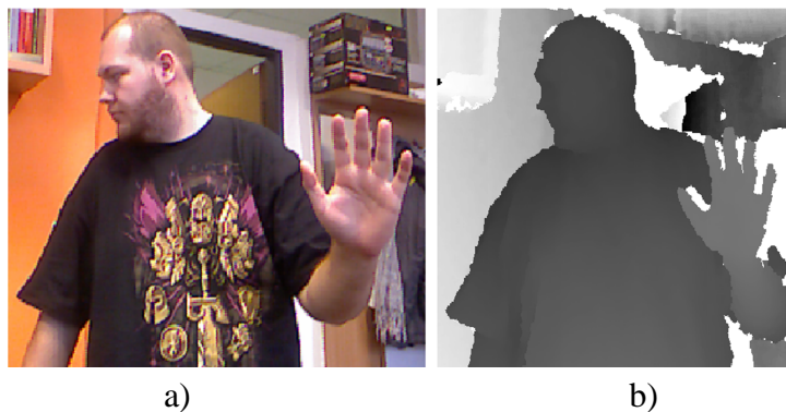
Fig. 3. Kinect sensor color image (a) and disparity map (b).
