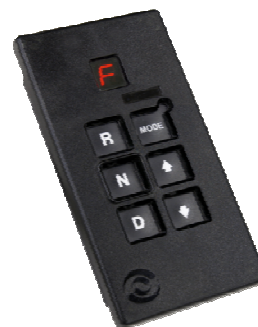
Fig. 7. The actual view of the PBSS selector fitted in the bus [2]
