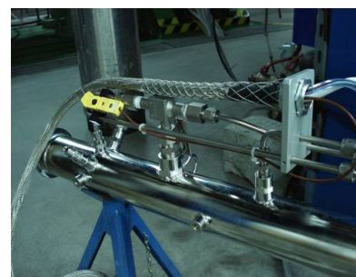
Fig. 3. Mass flow meter measuring the exhaust mass flow
