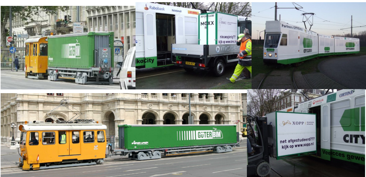
FIG. 4. The example of a tram and a universal tram wagon carrying swap-body in Vienna and specially modified Box in a trial operation in Amsterdam
