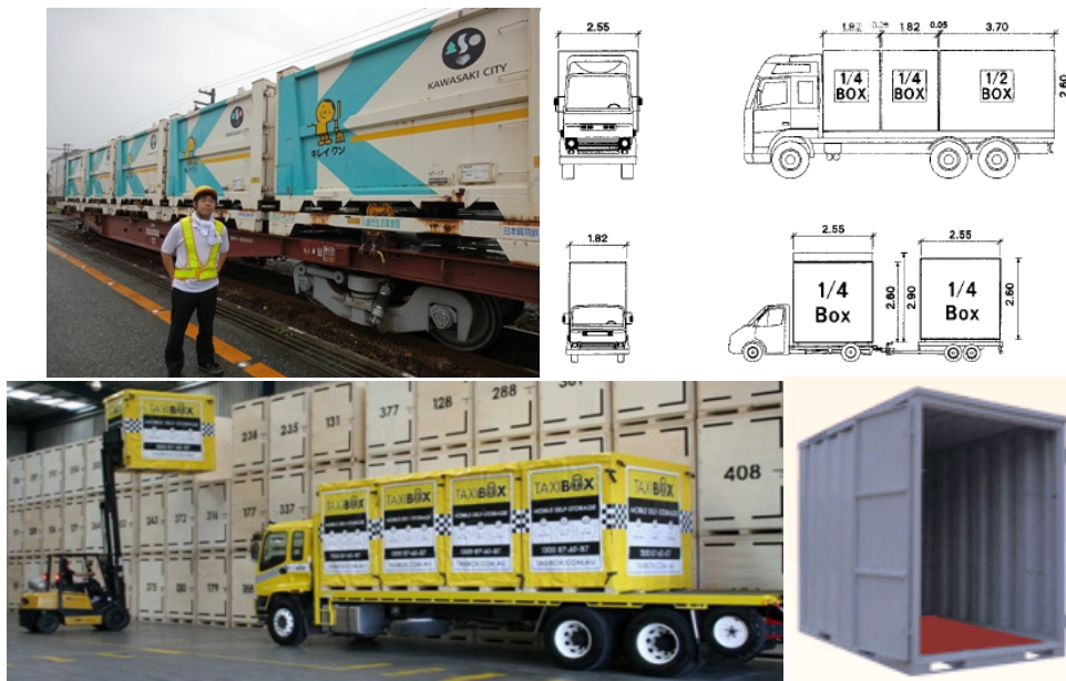
Fig.1. Example of small logistics box – on the right are small containers loaded at railway wagons in Japan and on the right proposed standardization of dimension lines in Europe; on the bottom from left to right – Australian taxibox and minibox – also known as mini container (ISO 10 ft. container).
