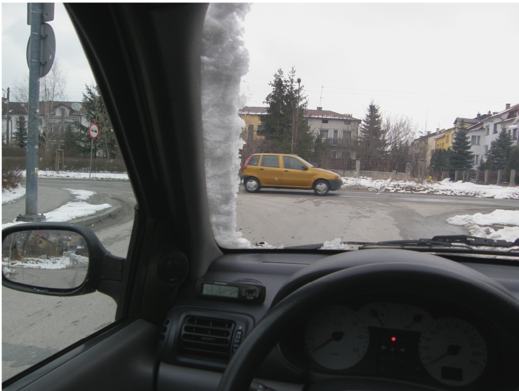
Fig. 2. The view from the car cab with the area not reached by a wiper blade.
