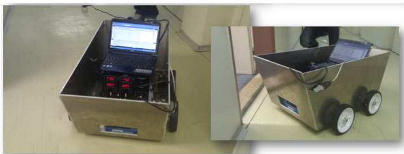
Fig. 5. The first version of a robotic chassis for outdoor measuring
