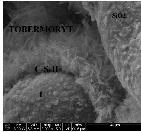
Fig. 2. The phase structure of a sand-lime product.
