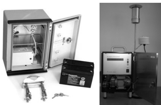
Fig. 2. Deviance for statistic of traffic driving Sierzega (left) and low-volume sampler Leckel LVS3 (right).
