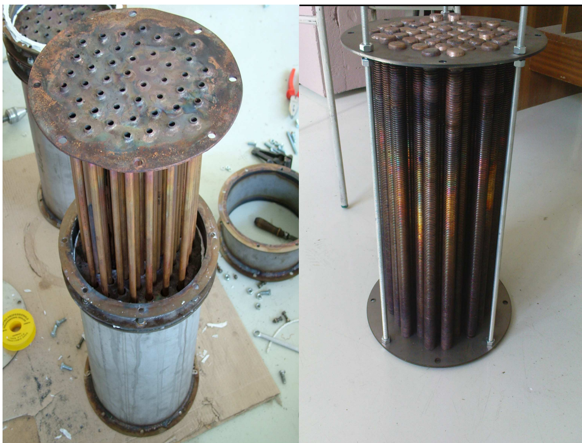
Fig. 3. Construction of adsorber
