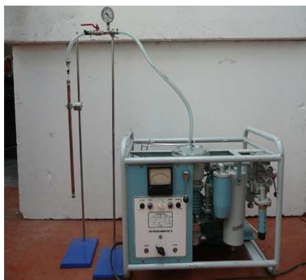
Fig. 2. Pumping air through a rotary pump
