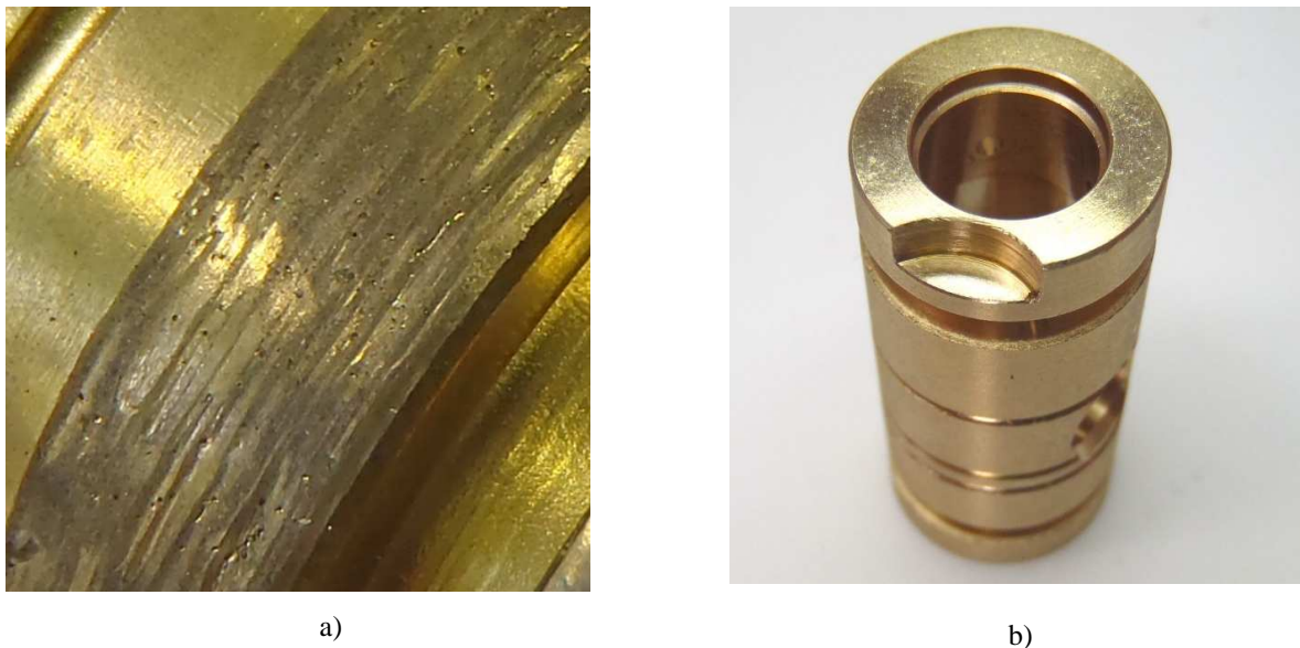
Fig. 4. Thrust bearing bush: a) outside surface (magnification 20x), b) new bearing bush (magnification 3x)
