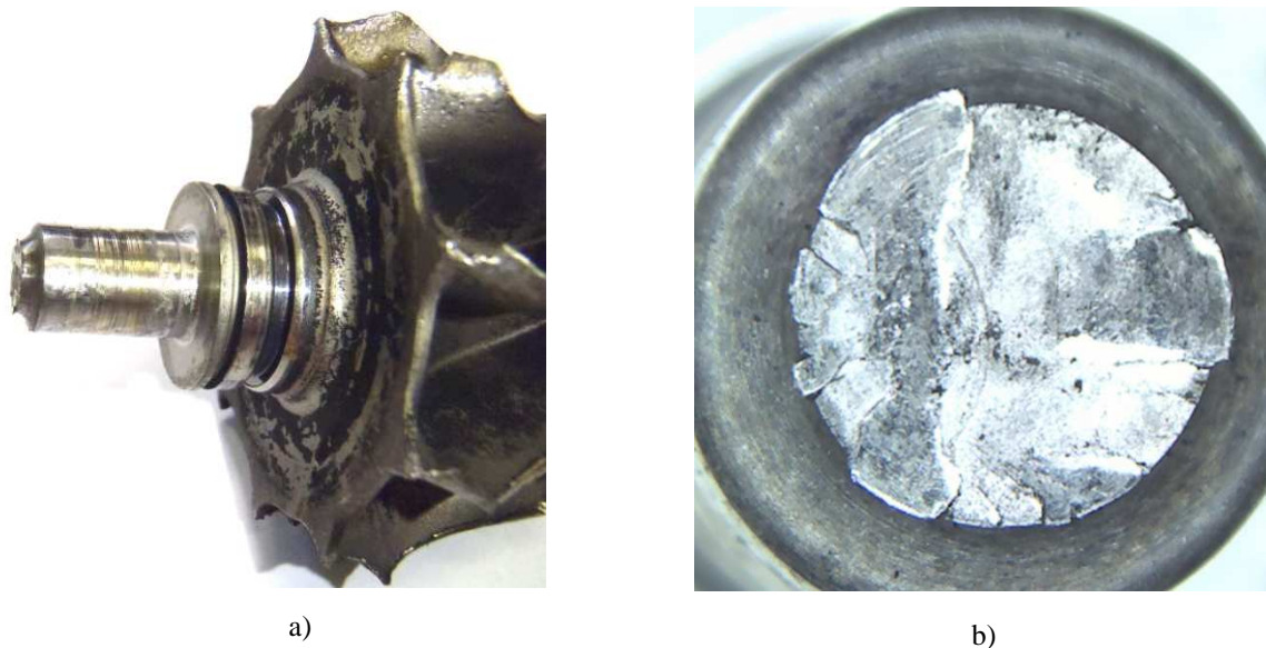
Fig. 5. The broken shaft: a) magnification 2x, b) magnification 10x
