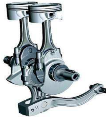
Fig. 2. Piston crank assembly in the Rotax-BMW engine [2]
