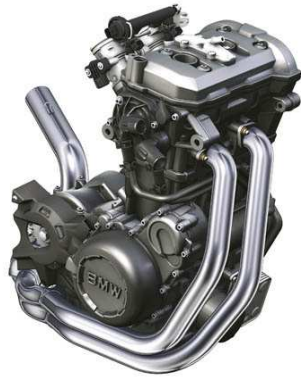
Fig. 1. Two cylinder Rotax-BMW engine, of displacement of 0,798 dm 3 and unit power output of 80 kW/dm 3 , used in BMW motorcycles [2]
