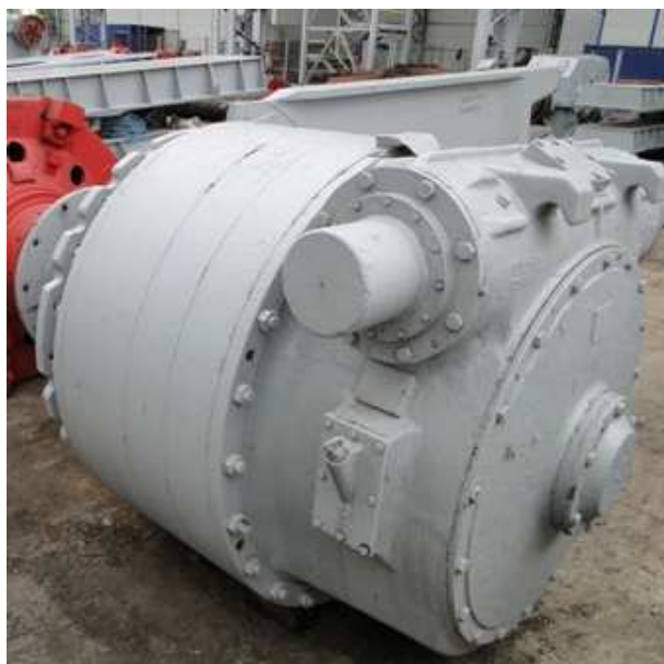
Fig. 1. High power transmission worm gear drive - motoreducer
