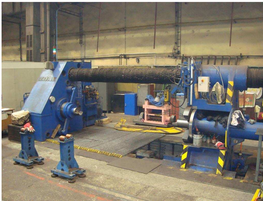
Fig. 4. The pressing machine for brake discs and monoblocks pressing
