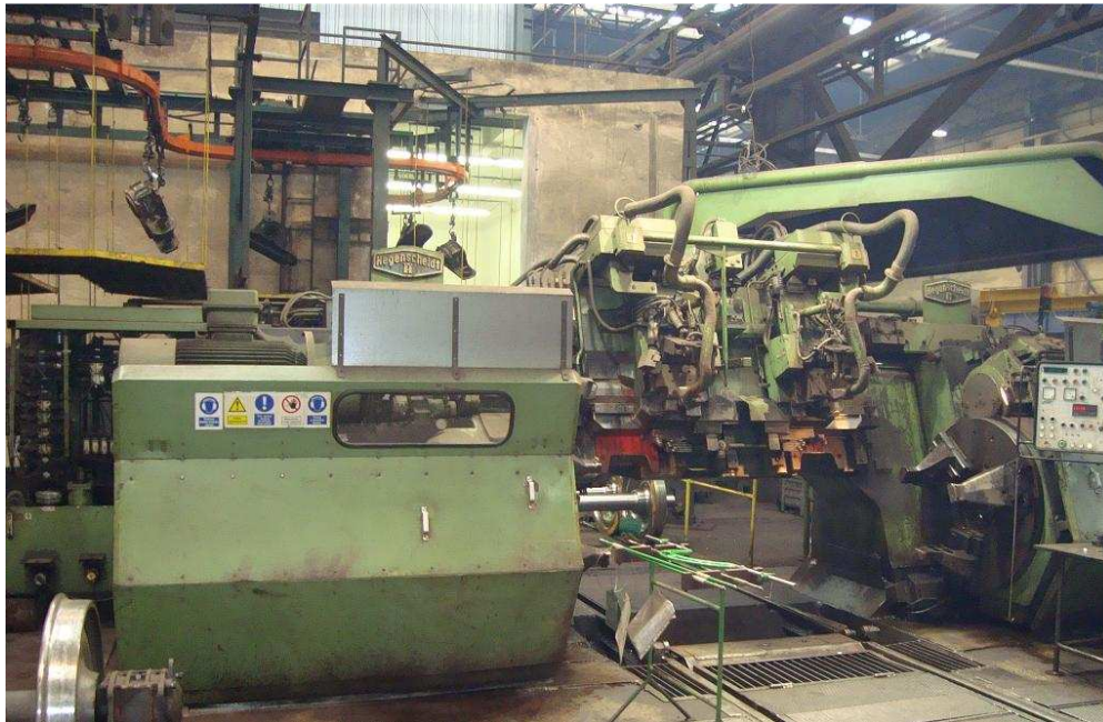
Fig. 2. Device for turning of the driving profile and the brake discs
