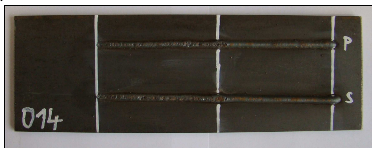
Fig. 2. Supply interruption of protective atmosphere. P – pulse transfer welding, S – dip transfer welding.
