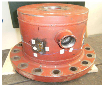
Fig. 5. Location of tensometers on drilling component.
