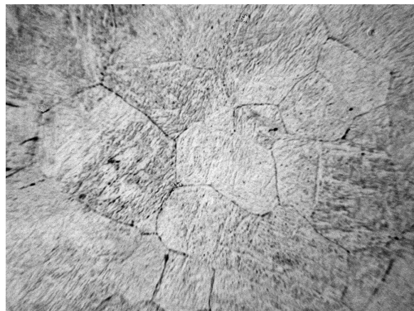
Fig. 2. The microstructure after quenching of X12Cr13 steel (500x)
