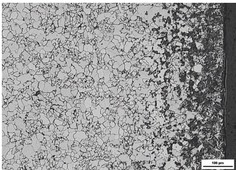
Fig. 2. Microstructure of HAZ. Steel EN ISO S235JR. Magnification: 100x. Etched Nital 3%. Laser cut.
