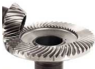
Parts of gearbox machined by method ISF
