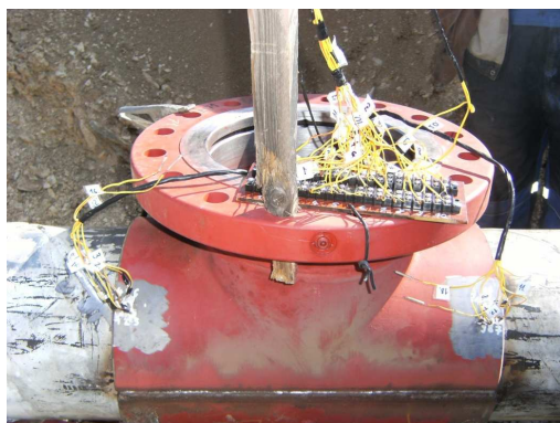
Fig. 3. Thermocouples located on fitting.
