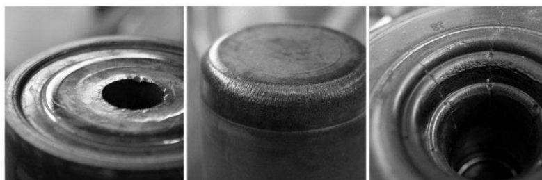
Fig. 1. Visualization of wear forging tool
