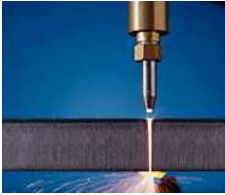
Fig. 1. Oxy – fuel cutting
