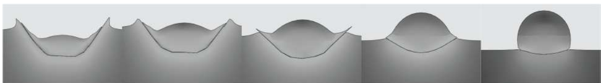
Fig. 4: Deformation of the particle after 0.5 and 1 ns considering different particle velocities
