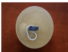
Fig. 2. The sample of investigated material in dentacryl.
