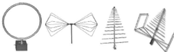
Fig. 2. Antennas used for the EMF measurements (from the left: loop antenna, biconical antenna, log-periodic antenna, biological antenna) [source: www.ahsystems.com]
