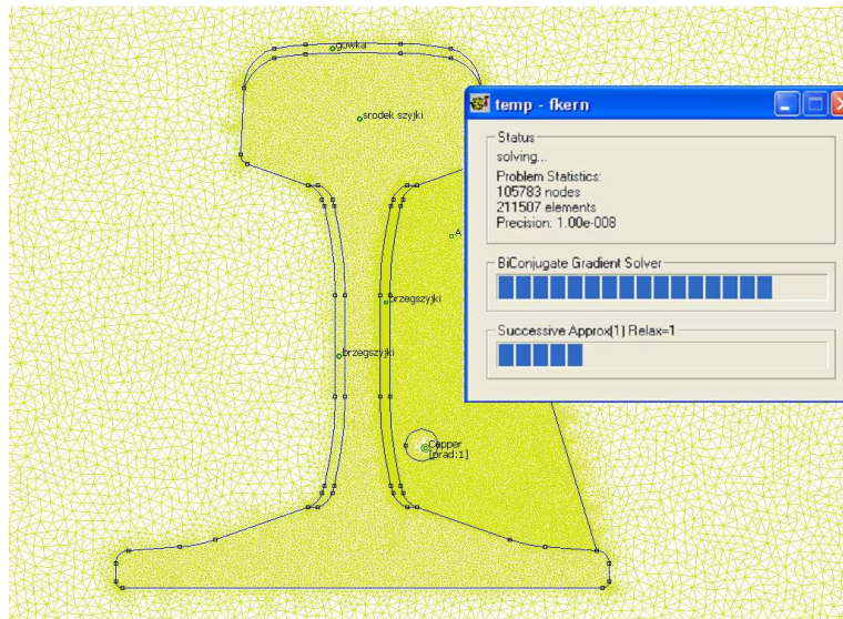
Fig.2. A simulation model of 60E1 (MES) rail in FEMM.
