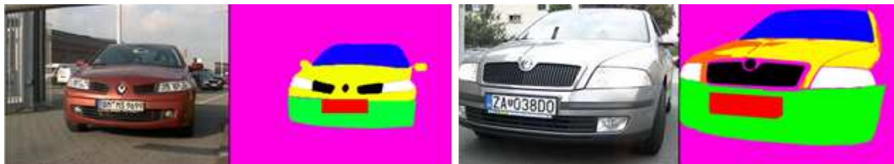
Fig. 1. Images of the distinctive areas shown on a vehicle. The picture on the left shows an ordinary car, with the bonnet at about 30% of the car area. The picture on the right illustrates problem of reflection. Here the color orange represents the true/original color of the car (about 5% of the area) and yellow covers the remaining bonnet area and depicts the reflective, not original color of the car (about 10% of the area).
