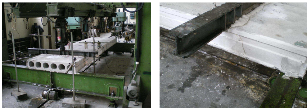
Fig. 5. Test configuration, shear failure of unit.
