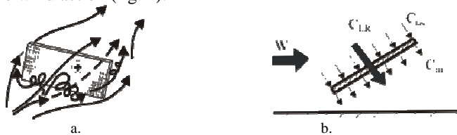
Fig. 2. The wind flow around a plate inclined with an angle from the wind direction, (a) and the elements of determination of coefficient c_{LR} , (b)
