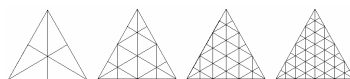
Fig.2. Consecutive face subdivisions using the second method of triangulation to generate regular octahedron-based polyhedra
