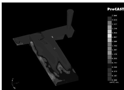
Fig. 4. Underpressure gating system with overpressure sprue..
