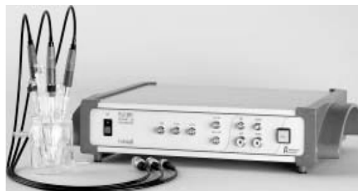
Fig.3 Experimental device used for assessing electrochemical properties (Voltalab 10)
