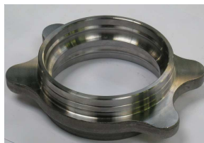
Fig. 1. Bearing ring applied in the experiments made of steel C56 E2
