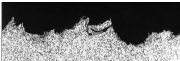
Fig.1 Section of sand shot peened surface of STN 41 1375.10 steel [4]
