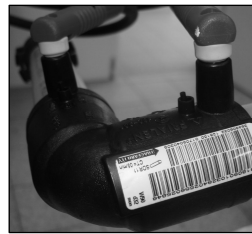
Fig. 6. Visual control weld through replacement pin welder indicator.
