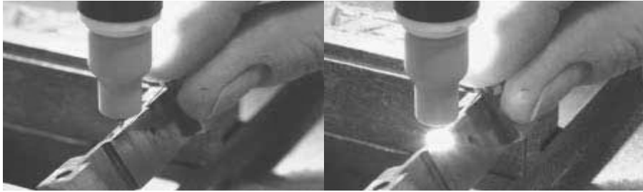
Fig.1. Method of melting-down of basic and additional material
