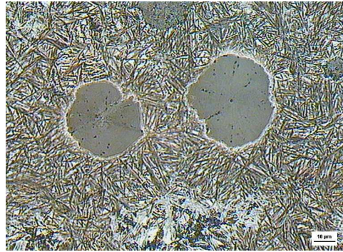
Fig. 4. Microstructure, ADI 250 °C / 240 min, mag. 500x, etch. Beraha-Martenzit
